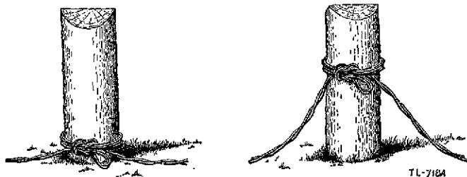
FIGURE 78.—Method of tying wire at ground level.
